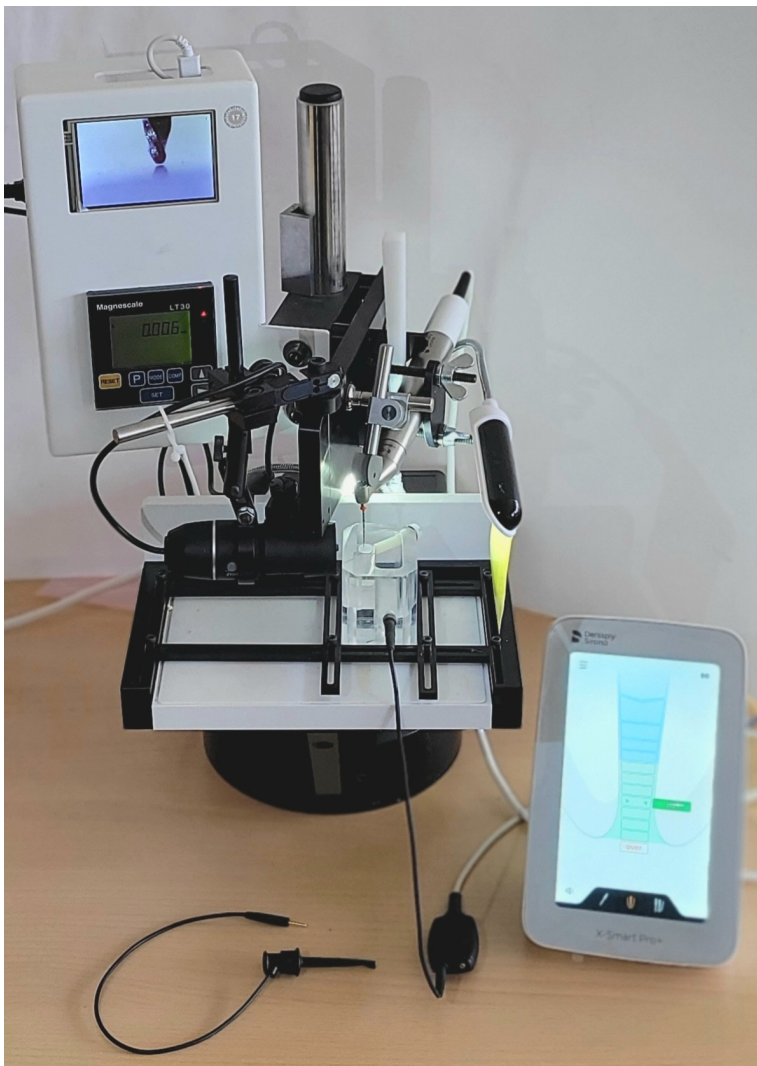
Figure 6: Bench test for the evaluation of the integrated apex location (without file clip).
