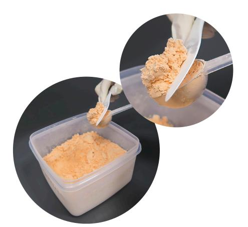
**3.** Scoop the powder from the container and remove any excess powder with a dry spatula.
