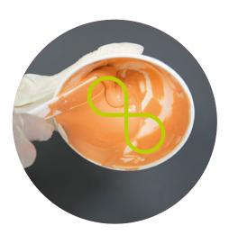
**6.** Mix the material with a figure-of-eight action and compress the material against the side of the mixing bowl in order to produce a smooth, bubble-free mixture.
