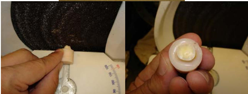
Embedding in acrylic – Preparation of flat surface
